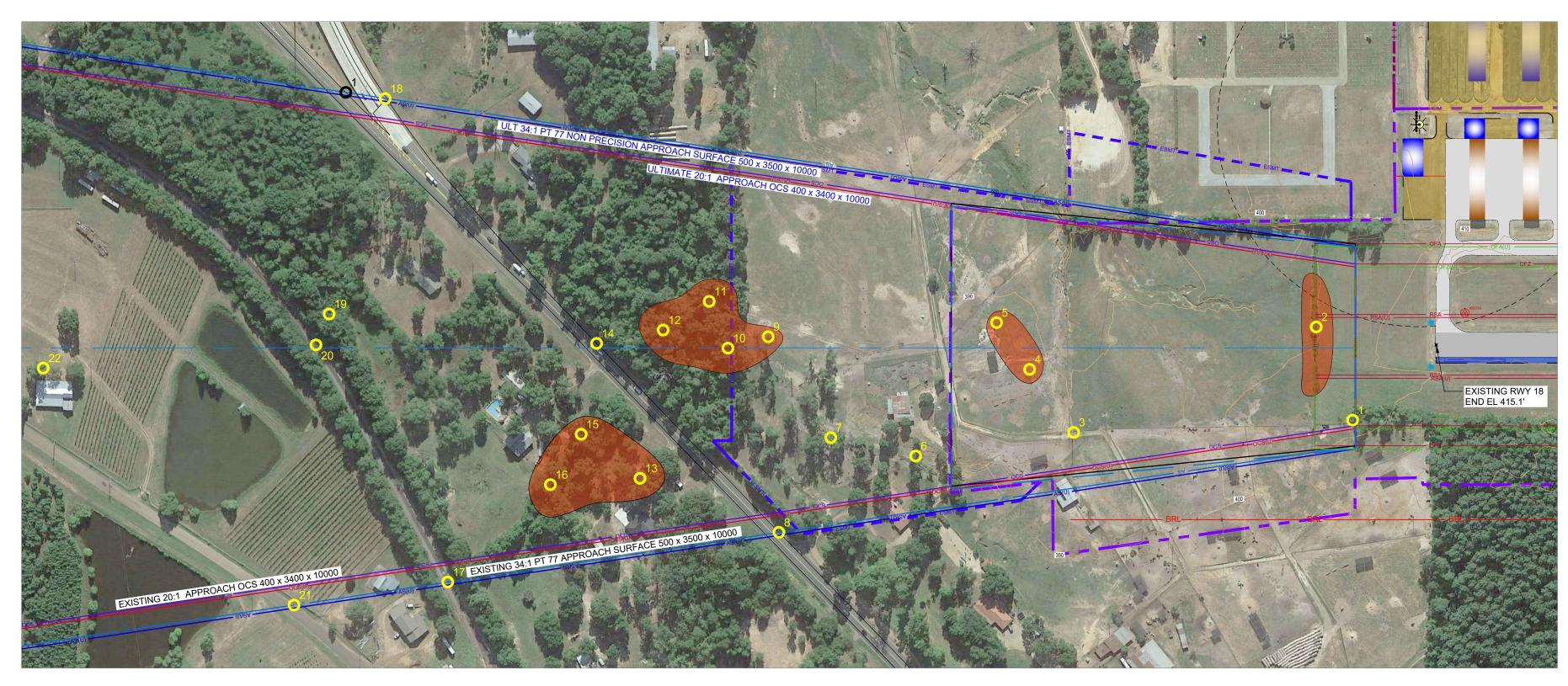
OBSTRUCTION ANALYSIS WAS DETERMINED USING BASEMAPPING PROVIDED BY TXDOT. A NEW OBSTRUCTION SURVEY WAS NOT CONDUCTED FOR THIS PROJECT. THERE MAY BE OBSTACLES NOT ACCOUNTED FOR DUE TO THE AGE OF THE SURVEY. BEST AVAILABLE INFORMATION WAS USED ACCORDING TO THE CONTRACT SCOPE.
